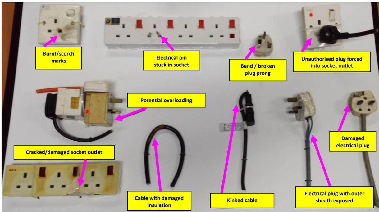
Figure 10: Examples of things to look out for during routine inspections
