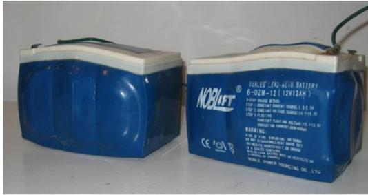
Figure 12: Bloated lead acid batteries
